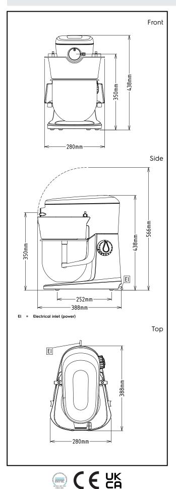
**Electric** 200-240 V/1N ph/50/60 Hz Supply voltage: **Total Watts:** 0.5 kW Capacity: Performance (up to): 0.75 kg/Cycle
